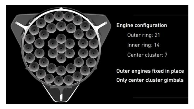
So, this uses 42 Raptor engines. It's a lot of engines, but we use nine on a Falcon 9, and with Falcon Heavy, which should launch early next year, there's 27 engines on the base. So we've got pretty good experience with having a large number of engines. It also gives us redundancy, so that if some of the engines fail, you can still continue the mission and be fine.
