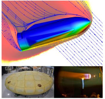
We've been refining the heat-shield technology using our Dragon spacecraft, and we're now on version three of PICA, which is "phenolic impregnated carbon ablator, " and it's getting more and more robust with each new version, with less ablation, more resistance, less need for refurbishment.
