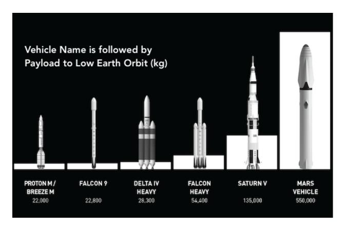
So this gives you a sense of vehicles by performance, so current and historic. I don't know if you can actually read that, but: In expendable mode the vehicle that we were proposing, we'd do about 550 tons, and about 300 tons in reusable mode. That compares to Saturn V's max capability of 135 tons.
