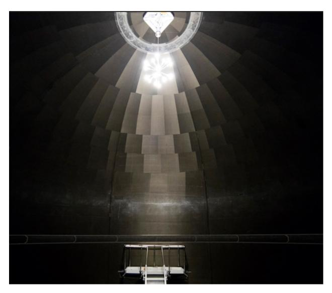
So you can get a real sense for how much, just how big this tank is. It's actually completely smooth on the inside, but the way that the carbon-fiber plys reflect the light makes it look faceted.
