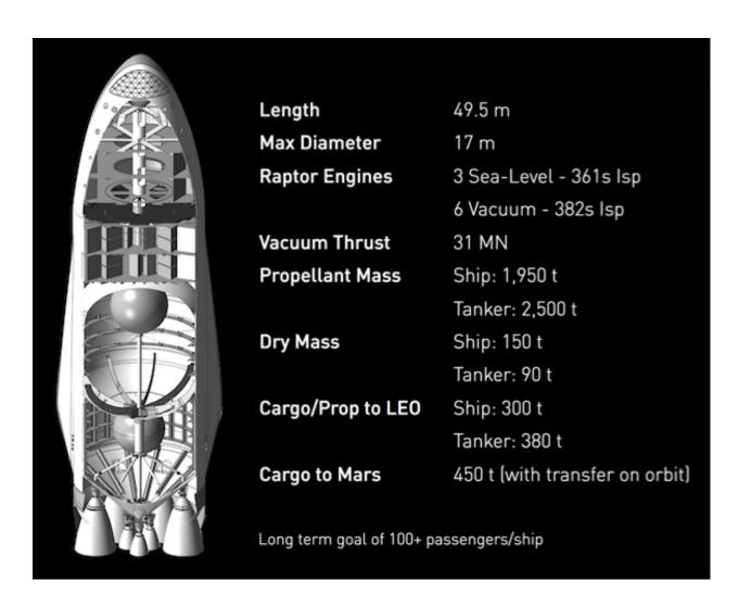
So for the spaceship itself, in the top we have the pressurized compartment — and I'll show you a fly-through of that in a moment — and beneath that is where we would have the unpressurized cargo, which will be really flat-packed, in a very dense format. And below that is the liquid oxygen tank.
